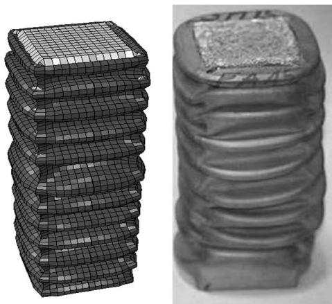
Fig5.. Comparison of experimental deformation [22] with numerical prediction.
