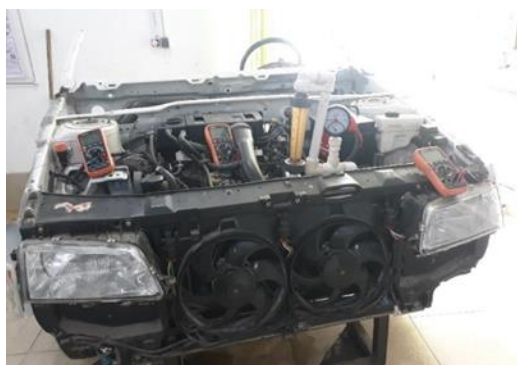
Figure 8: Measuring equipment installed on the XU7 engine
