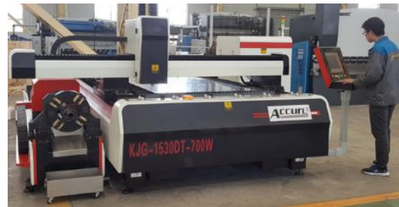
Figure 1: ACCURL laser tube cutting machine in operation
