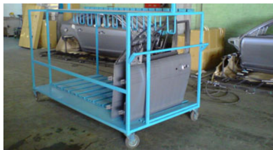
Fig. 1. Mobile material handling shelf
