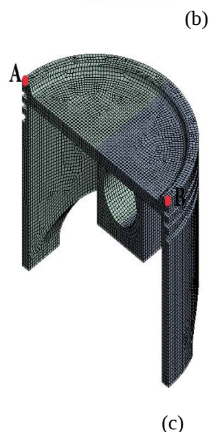
Figure 1. The piston used in the FE analyses: a) gasoline engine b) the piston, c) meshing of the FE model.
