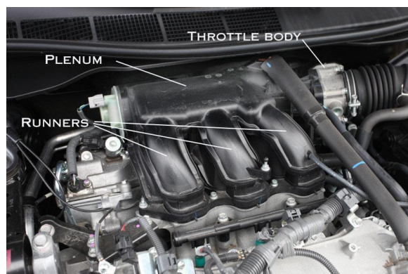
Figure 2: The location of geometric parameters studied in manifold analysis
