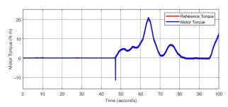
Figure 21: Upper and Lower limits of Torque Hysteresis controllers are set to 0.6885 and (-0.918) respectively.
