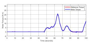
Figure 27: Upper and Lower limits of Torque Hysteresis controllers are set to 0.459 and (-0.459) respectively.
