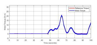
Figure 23: Upper and Lower limits of Torque Hysteresis controllers are set to 0.918 and (-0.459) respectively.
