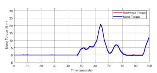
Figure 26: Upper and Lower limits of Torque Hysteresis controllers are set to 0.459 and (-0.918) respectively.
