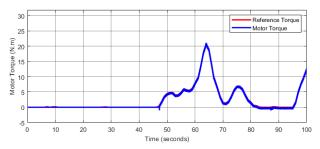
Figure 20: Upper and Lower limits of Torque Hysteresis controllers are set to 0.6885 and (-0.459) respectively.
