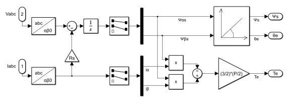
Figure 2:Estimator model developed in MATLAB Simulink environment.
