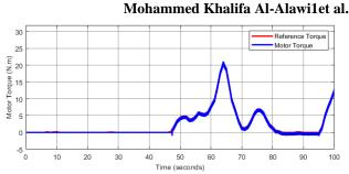
Figure 24: Upper and Lower limits of Torque Hysteresis controllers are set to 0.918 and (-0.6885) respectively.
