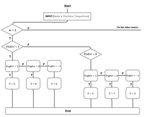
Figure 6:Algorithm flowchart of vector selection technique.
