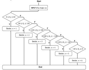
Figure 5:Algorithm flowchart of sector selection technique.
