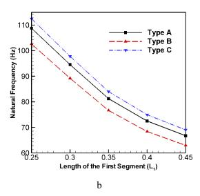
**Figure 4:** Variation of the natural frequency of clamped folded plates versus first segment length for various porous distributions, a)n=1 and b)n=2  $(L_1 + L_2 = 0.5 \text{m}, b = 0.2 \text{m}, h = 1 \text{mm}, m = 1)$
