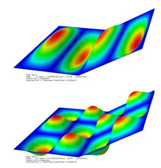
**Figure 2:** Two mode shapes obtained from Abaqus software
