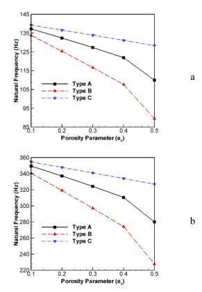
Figure 3: Variation of the natural frequency of clamped folded plates in relation to porosity parameters across various porous distributions, a)n=1 and b)n=2 ( $L_1 = L_2 = 0.5 \text{m}$ , b = 0.2 m, h = 1 mm, m = 1)
