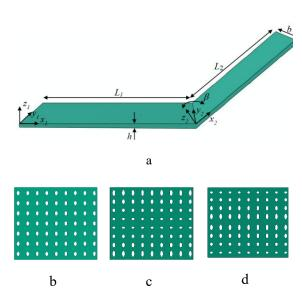
Figure 1: a) A depiction of a folded plate integrated with FG porous material and three types of porosity distribution along thickness, b)Type A, c)Type B and d)Type C
